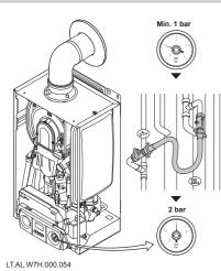
Check the boiler water pressure. If the water pressure is less than 1 bar, the system has to be topped up with
